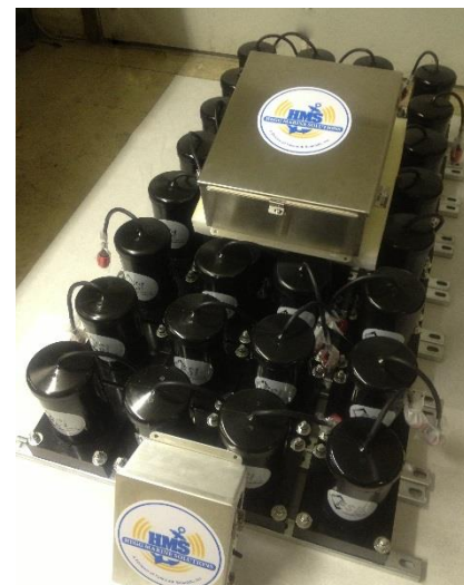
LF Transducer Array With Hull Mount J-Boxes & Amps
