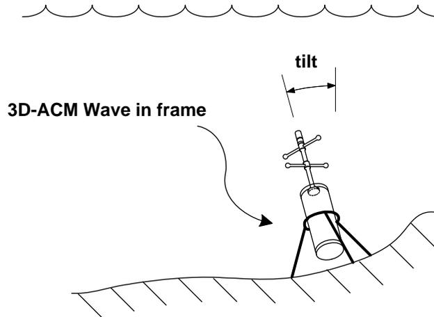
**Figure 3** *3D-ACM Wave positioning*
