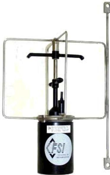
**Figure 4** *The 2D-ACM instrument with the protective frame*
