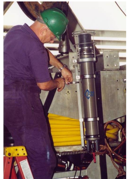
The USS-110 can be ROV-deployed or hand-mounted
