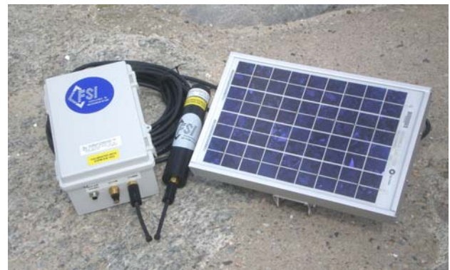
Tide Monitoring System with Optional Solar Charger
