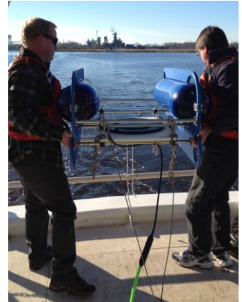
HMS-620 Source vehicle is compact and easy to deploy by hand
