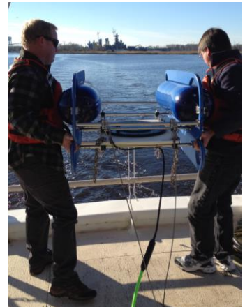
HMS-620 Source vehicle is compact and easy to deploy by hand
