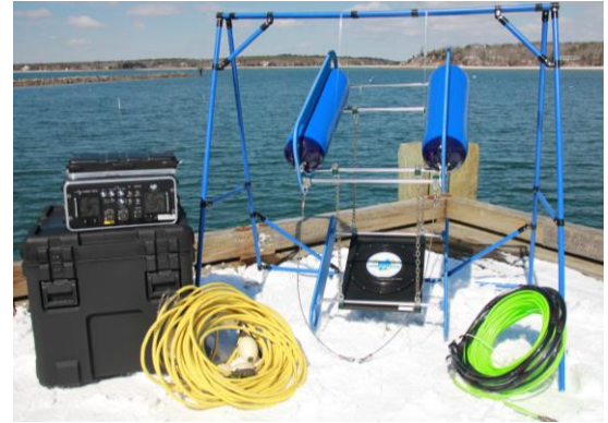
The complete Single-Source Bubble Gun™ System includes transceiver, shipping case, tow cable, hydrophone streamer, and source vehicle (suspended on display frame)
