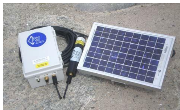
Tide Monitoring System with Optional Solar Charger
